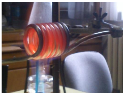
Figure 54: The spiral made from the copper tube at red glow
