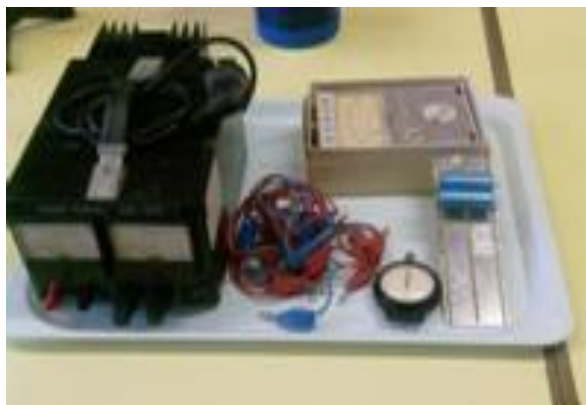
Figure 30: Equipment to study how voltage changes when we discharge a capacitor
