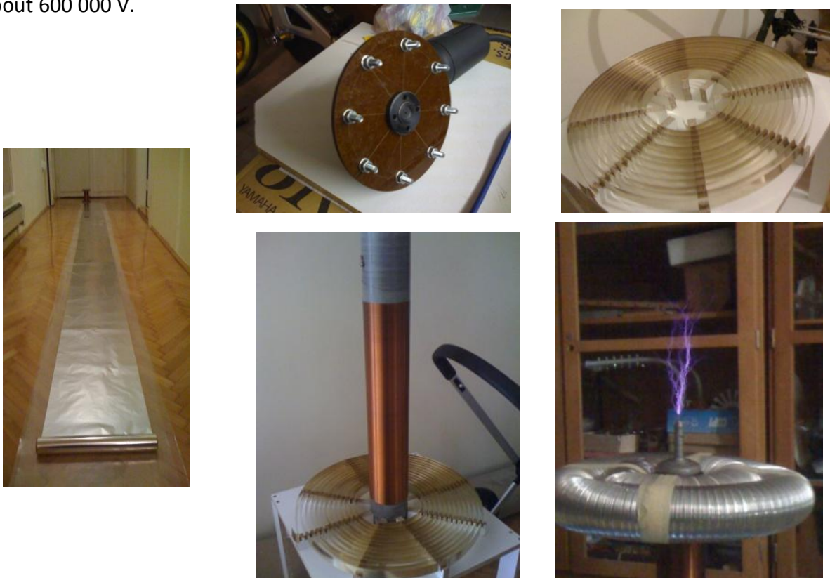
Figure 44: Making our spark-gap, capacitor, 13 loops of brass band, toroid, roof capacitance
