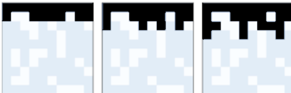
Figure 19: The first three time steps of generating a percolation fractal
