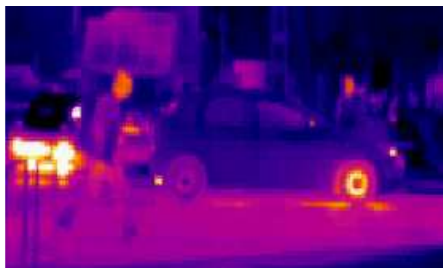
Figure 14. Thermopicture of a car with warm front disc brakes
