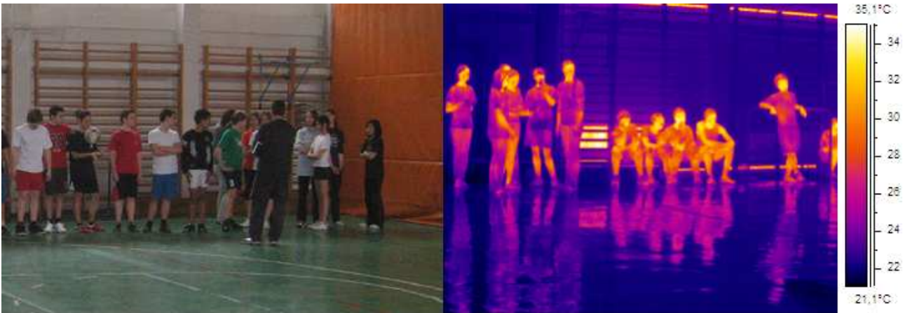
Figure 11. The matt linoleum cover of the floor behaves as a plan heat mirror in the gymnasium
