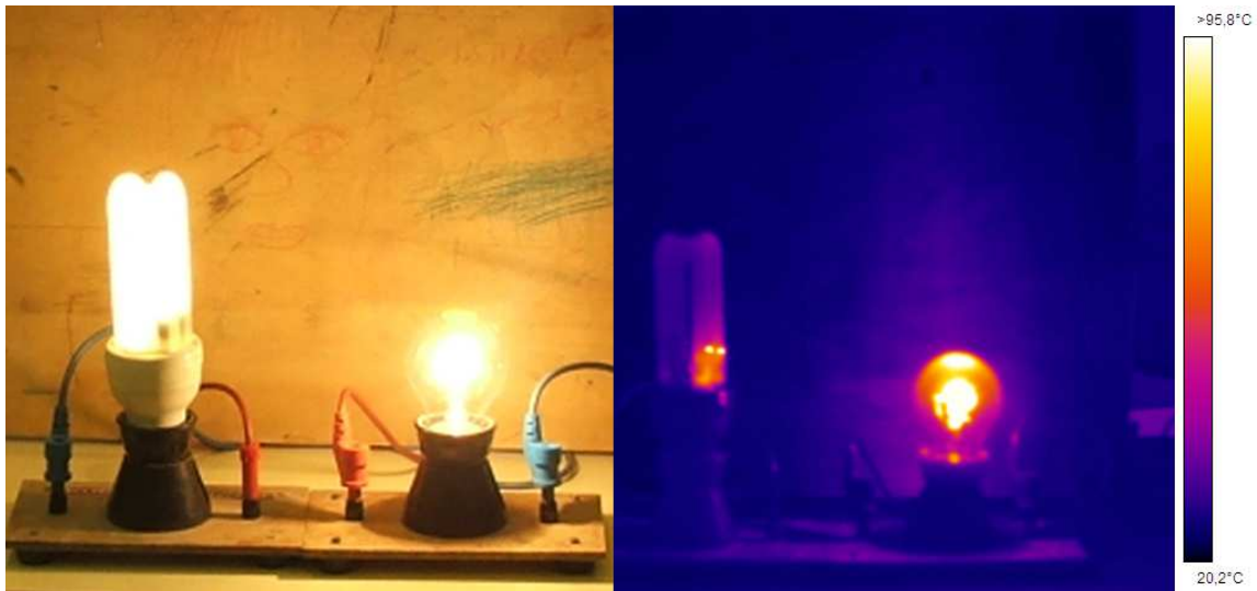
Figure 5. An energy saving and a traditional bulb in visible (left) and in infrared (right) light
