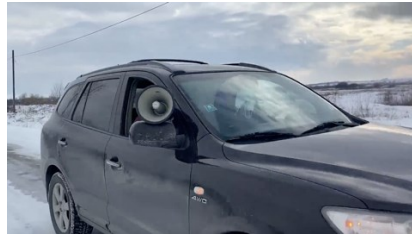
FIGURE 1. The sound source: a mobile phone with a tone generator and a loudspeaker placed on a moving car
