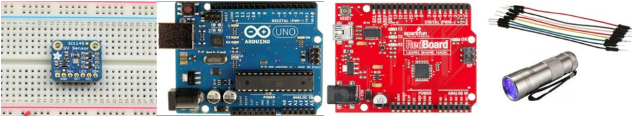
FIGURE 1. The breadboard, Si1145 sensor, Arduino and Redboard, UV lamp and wires for light and UV measurements
